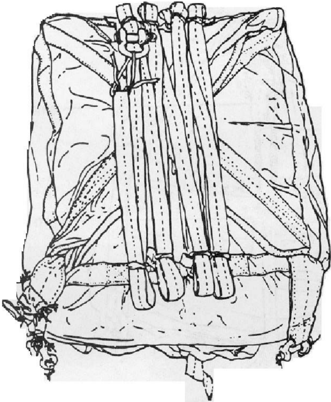
Figure 3-15 Static line stowage completed
